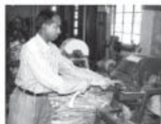
Fig. 2. Sisal fibre extraction with Raspador
